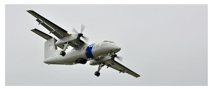
The Bombardier DHC-8 is a fixed-wing, medium -range multi-role patrol aircraft equipped with multimode radar and electro-optical/infrared sensors that can detect and monitor maritime and surface targets. Video recorders document suspect activities for evidentiary use. The DHC-8 is well suited to accomplish the mission of detecting, disrupting, and interdicting maritime smuggling.
