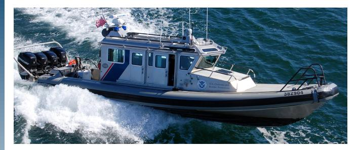
The 38-foot Secure Around Flotation Equipped (SAFE) Boat is used by U.S. Custom and Border Protection, Air and Marine Operations (AMO) for the pursuit and boarding (inland and offshore) of vessels transiting in locations with extreme weather conditions.
