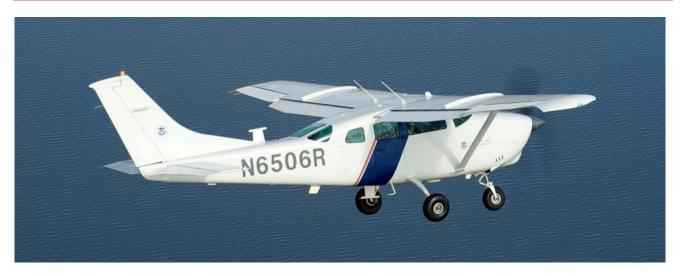
Cessna C206H and T206H "Stationairs" are high-wing, single-engine Light Enforcement Aircraft used by U.S. Customs and Border Protection, Air and Marine Operations (AMO) to support investigative and enforcement efforts by conducting surveillance, tracking and reconnaissance.
