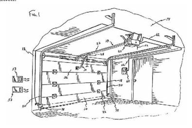
Compl. Ex. A, at 4, Sept. 13, 2018, ECF No. 4–1 ("319 Patent"). The motor drive unit, which opens and closes the garage door, contains a microcontroller (or controller) that is connected to the wall console "by means of a digital data bus." Id. at 23.
