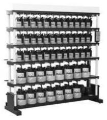
Each metal shelving unit comes equipped with a gear drive on the top of the shelf and safety guards on the bottom of the shelf. The safety guards lock the paint cans into place and secure them during mixing. A mixing shelf cover is also included to cover the gear drive and set additional paint cans on top of the shelving unit. A picture of the metal shelving unit and its components is provided below:
