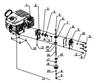
During oral argument, the Government clarified that Commerce determined that items 1 through 19 make up the modified vertical shaft engine, with item 1 (the engine) plus items 2 to 19 (the gearbox) comprising one single engine unit. Oral Arg. at 49:55–50:15. Plaintiff contended, on the other hand, that item 1 was the only engine unit and constituted a horizontal shaft engine, and items 2 to 19 (the gearbox) were not part of the engine. *Id.* at 11:57–14:58.
