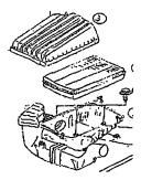
The function of this item is to clean the air within a vehicle engine.
